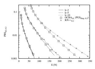
Figure 31: Efficiency of  $\mathcal{OCBA}_{LL}$  and  $\mathcal{KN}++$  depends on  $n_0$  (RPI1,  $k=5, \eta=1, b=100$ ).
